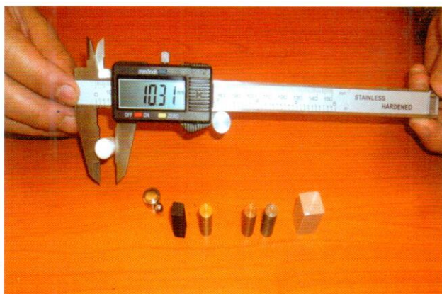
Figure 1.1: Vernier Caliper is used to measure diameter in mm.
